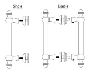
2. Loosen or remove set screws
